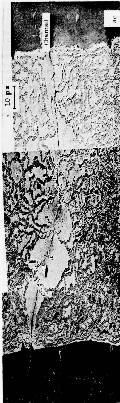
Figure 17. Electron Micrograph of the Necked-Down Film Region After ac Activation (X = 1152)
