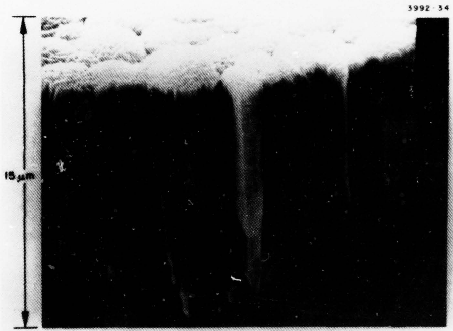
Figure 53. Typical SEM micrograph of tapered crystallite cross-sectional microstructure of CdS films.
