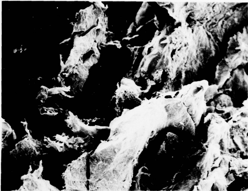
Fig. 20a. (110X) SEM: Fractured BBB Disc Pressed @ 475°C, 20 min
