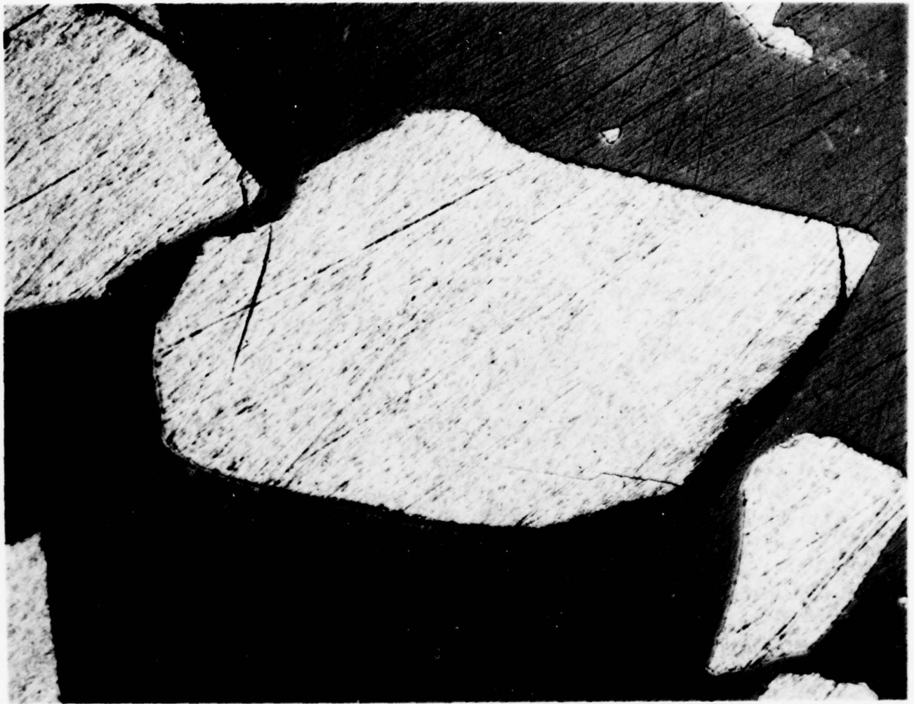
Fig. 4. (200X) Optical Micrograph: Co-precipitated BBB/PBI
