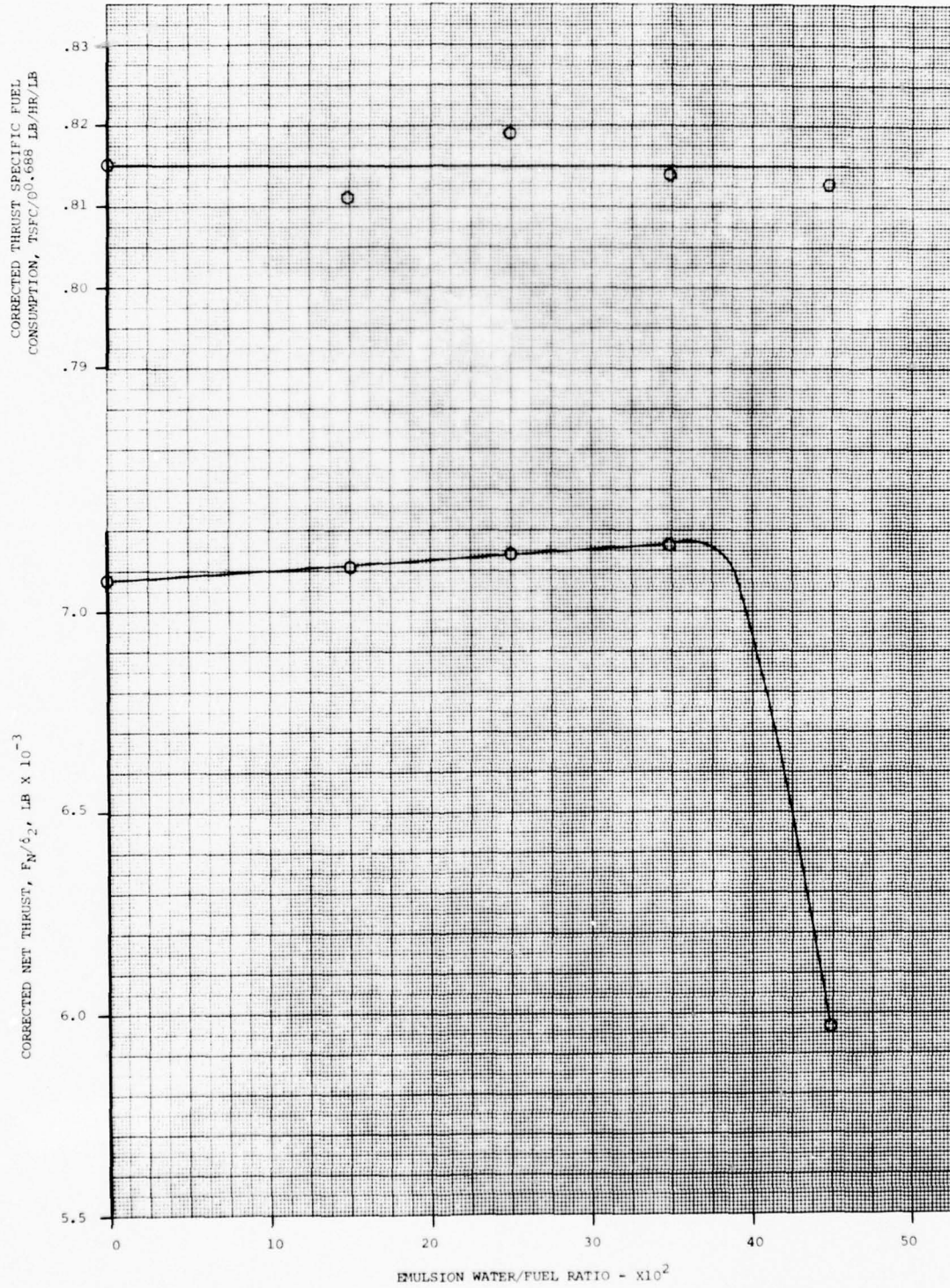
FIGURE 6. EFFECT OF WATER CONCENTRATION ON ENGINE PERFORMANCE AT PART POWER (57° PLA) AT T_2 = 75^\circ WITH MPC SPECIFIC GRAVITY SETTING OF 0.82
