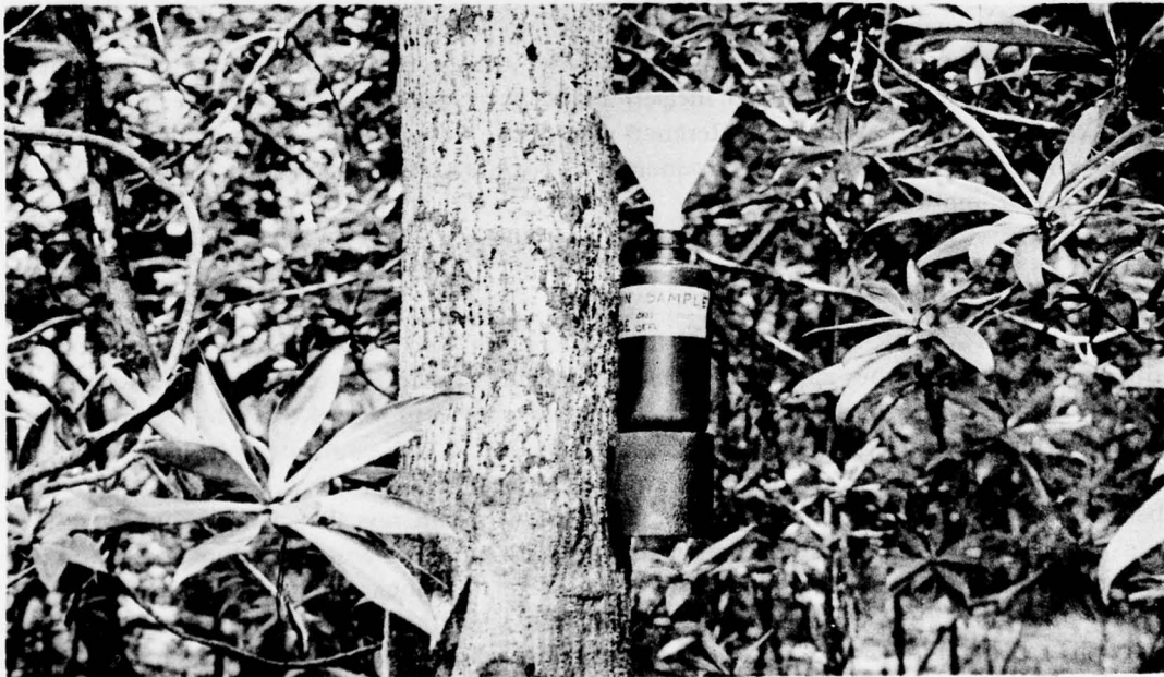
b. Close-Up of Funnel/Bucket Collection System.
