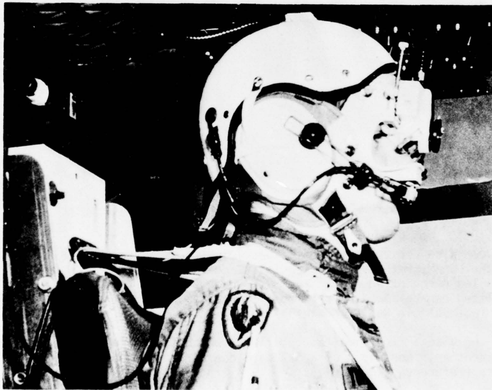
Figure 1. Aviator Wearing the Modified NAC Eye Mark Recorder
