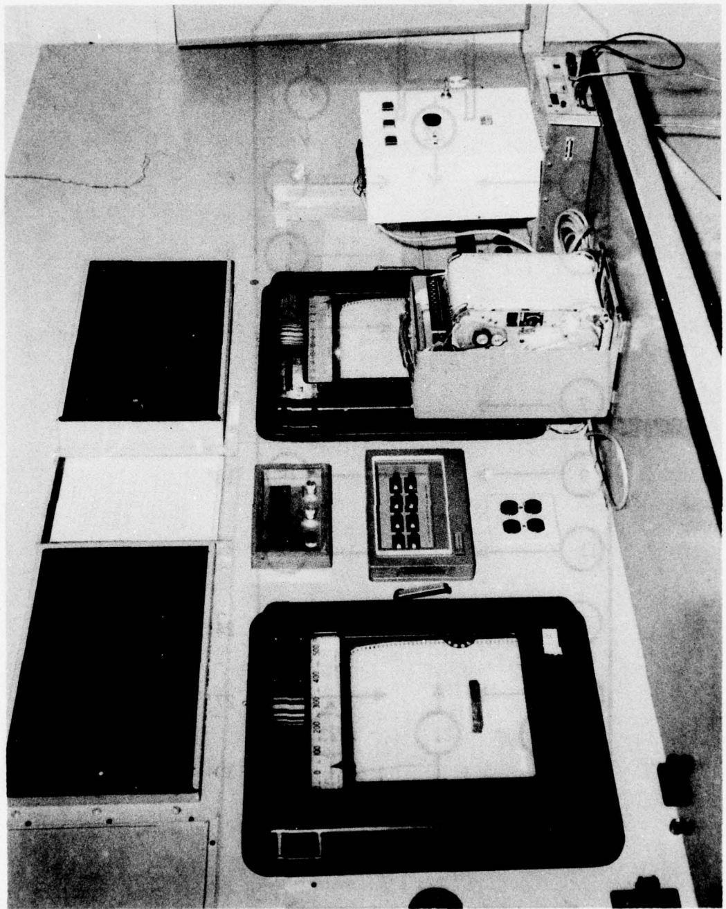
Figure 11. Environmental chamber temperature and alarm monitoring instrumentation.
