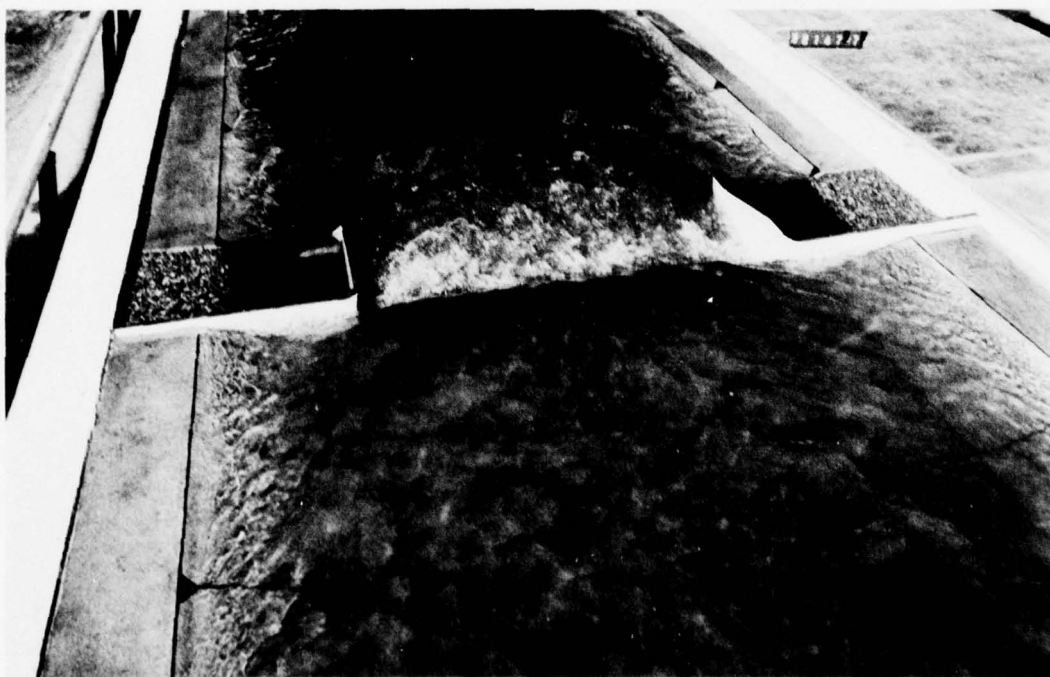
b. Tailwater el 82.1 (0.9 ft below rating curve); forced hydraulic jump
