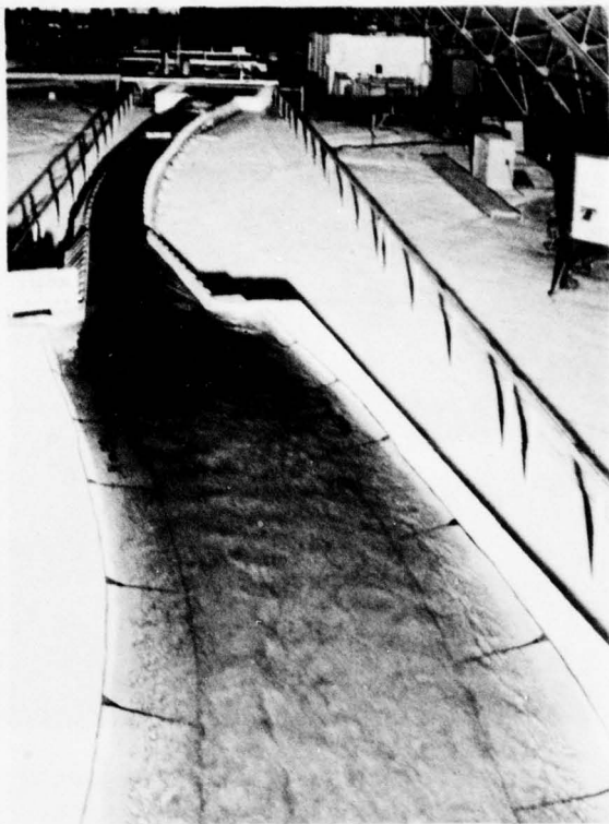
Photo 11. Overall view of model (Bucana Channel, orig- inal design); design flow 28,900 cfs
