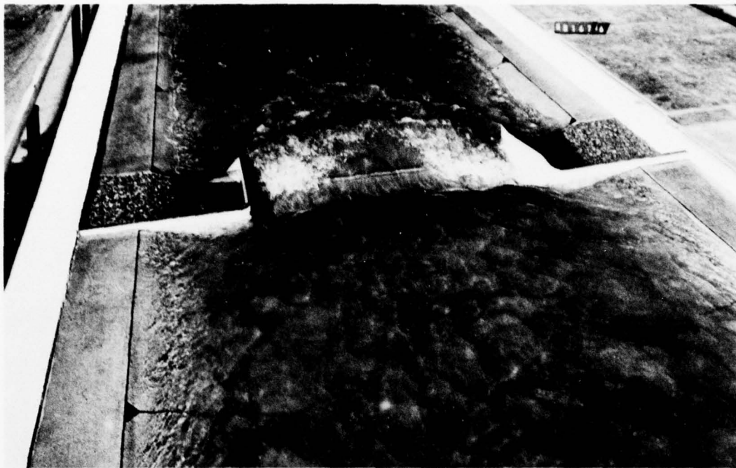
a. Tailwater el 81.2 (1.8 ft below rating curve); hydraulic jump is sweeping out of drop structure
