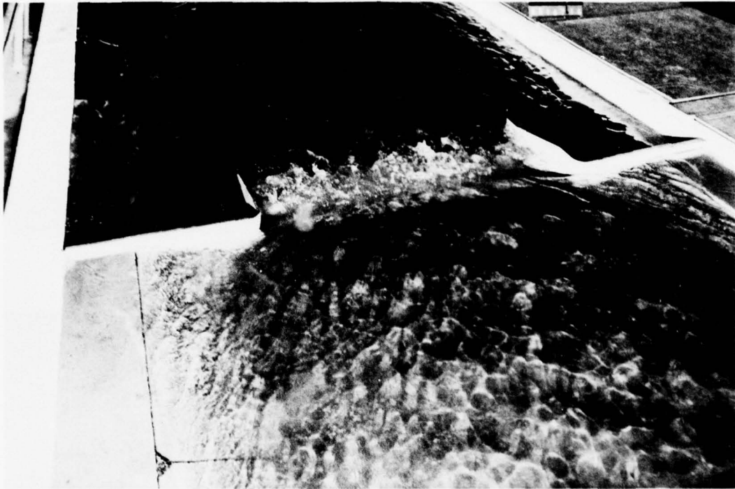
c. Tailwater el 108.6, submerged jump
