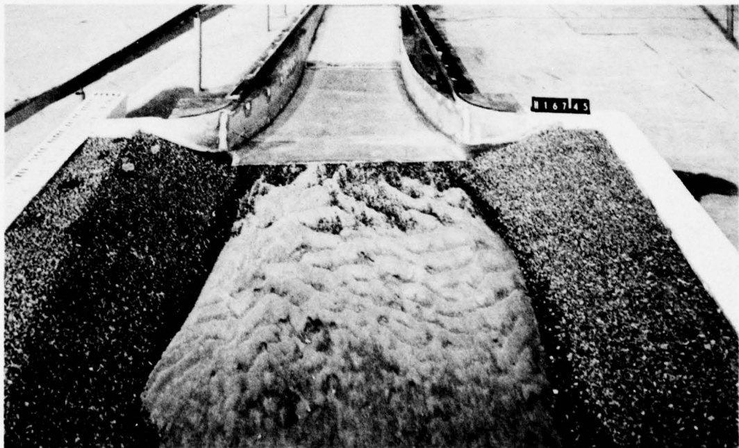
Photo 23. Original riprap plan after 30-min (prototype) operation with design flow 28,900 cfs, Bucana transition design 3
