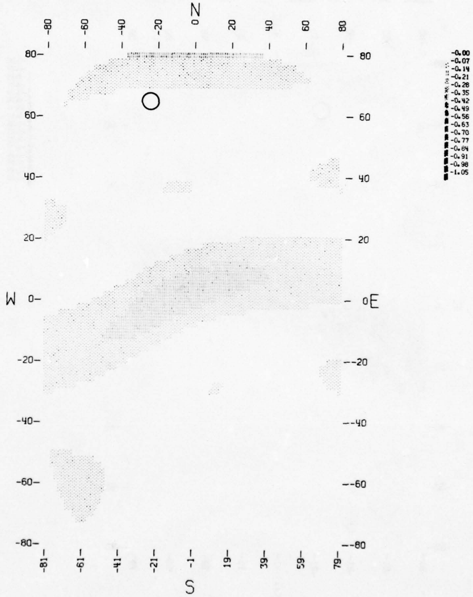
Fig. 41 - Scintillation index map (sunspot number = 0; summer). The center of the circle is the approximate location of Keflavik, Iceland (23°W, 65°N).
