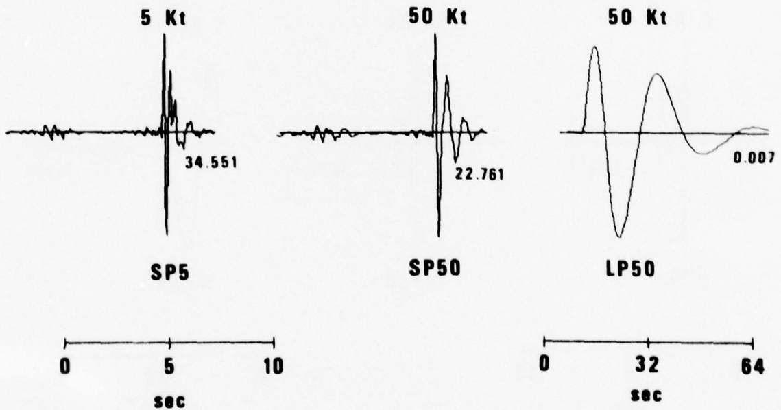
Figure 8. Crustal frequency response function, shown as linear power spectrum of the receiver crustal impulse response, receiver crust impulse responses, synthetic seismograms for the LRSM station FK-CO. The numbers to the right of abscissa indicate the maximum power or amplitude as appropriate.
