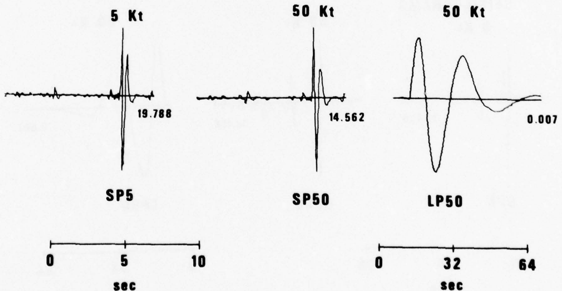
Figure 12. Crustal frequency response function, shown as linear power spectrum of the receiver crustal impulse response, receiver crust impulse responses, synthetic seismograms for the LRSM station HN-ME. The numbers to the right of abscissa indicate the maximum power or amplitude as appropriate.
