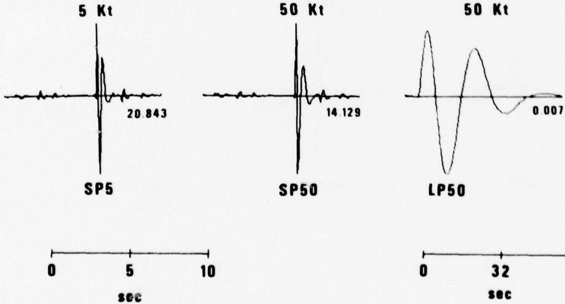
Figure 7. Crustal frequency response function, shown as linear power spectrum of the receiver crustal impulse response, receiver crust impulse responses, synthetic seismograms for the LRSM station DR-CO. The numbers to the right of abscissa indicate the maximum power or amplitude as appropriate.
