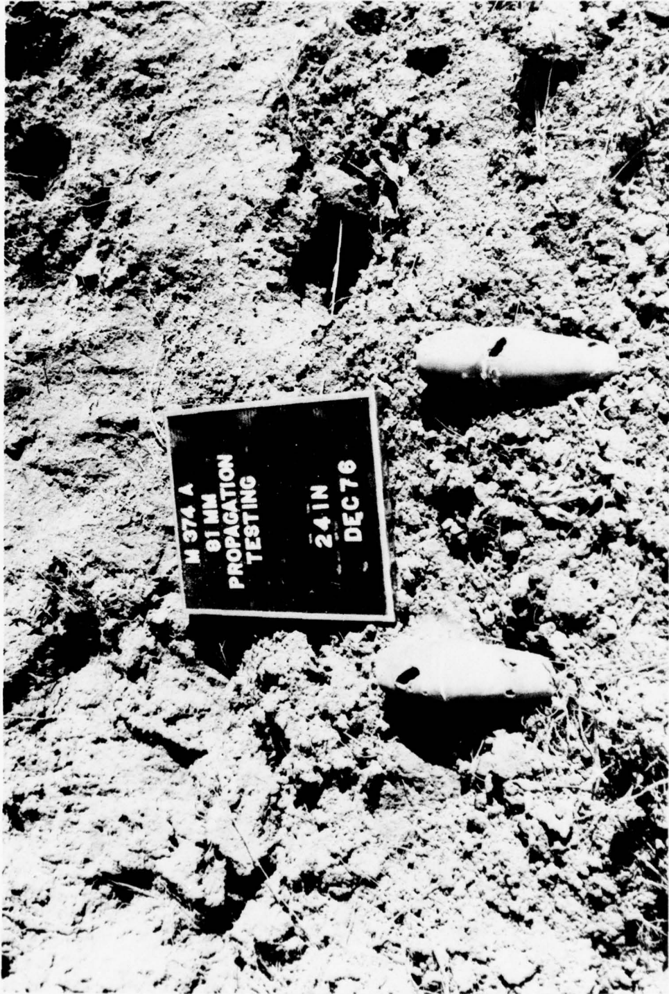
Fig 9 Single projectile post-test results showing typical acceptors at the 24-inch safe separation distance
