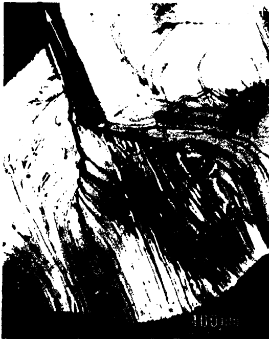
Fig. 14. Fractograph (optical) of cadmium after fracture in liquid gallium showing 'river lines' on a cleavage-like facet.
