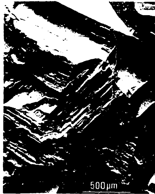
Fig. 13. Fractograph (SEM) of cadmium after fracture in liquid gallium showing 'flat' cleavage-like and brittle-intercrystalline facets.
