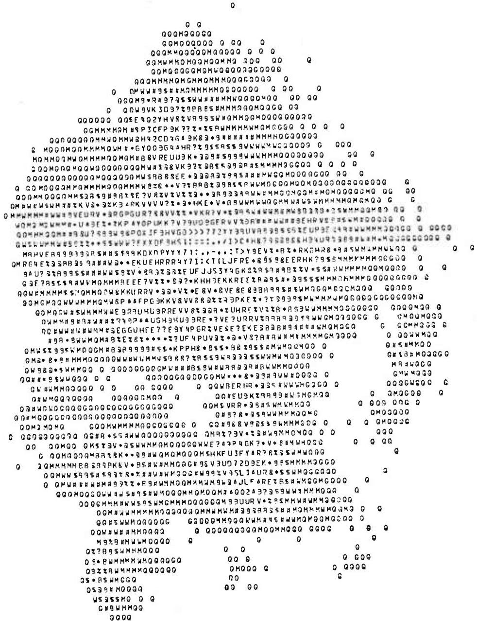
Figure 8-Energy Level Distribution in a Reflected Laser Spot
