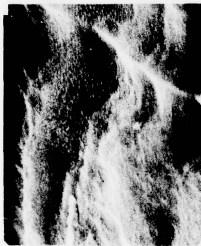
Figure 16 SEM Photomicrograph -- Anodized at 100°F -- 2024-T3 Clad
