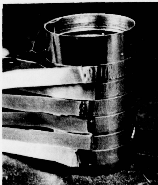
(b) Specimen For Environmental Exposure - Three Strips to Be Tested After 60 Days and Three After 120 Days Exposure
