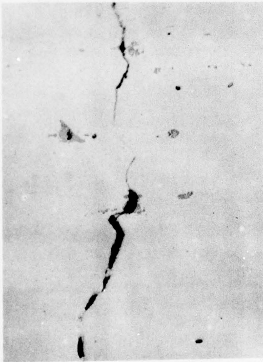
Figure 69 - Optical micrographs taken along the crack front at short crack length in the High Cu 7475-type alloy. Crack propagation direction is into the plane of the paper. 500X As-Polished
