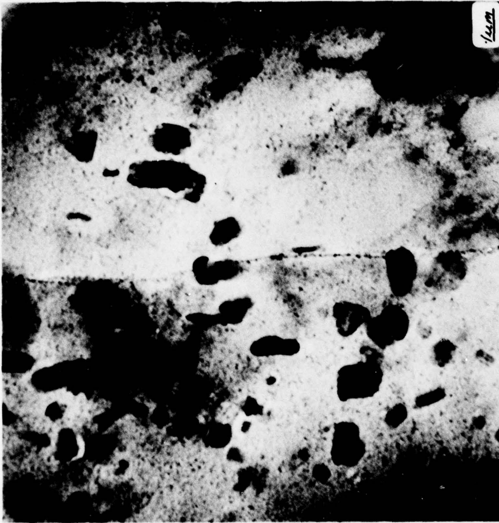
Figure 22 - Bright field micrograph of 7075-T6 showing the size and distribution of E-phase ( Al_{12}Mg_2Cr ).
