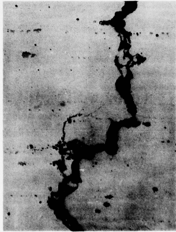
Figure 70 - Optical micrographs taken along the crack front at long crack length in the High Cu 7075-type alloy. Crack propagation direction is into the plane of the paper. 500X As-Polished
