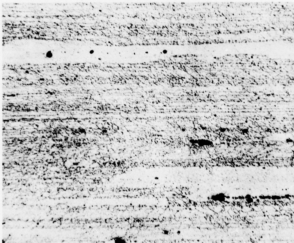
Figure 16 - Longitudinal section of a. 7050 (454543) and b. Higher Cu 7475-Type (454546) showing the differences between similar alloys containing Zr or Cr. (Hot HNO 3 Etch, 500X)
