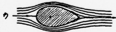
Figure A-1. Theoretical and Actual Flow Patterns around Spheres and Aerodynamically-Shaped Bodies.
