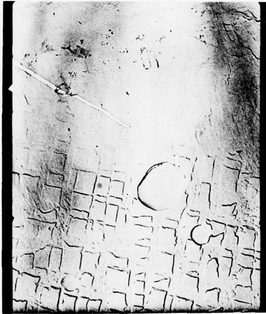
Figure 7. Replica of Superalloy AF2-1DA Showing Slip Plane. 12,000x
