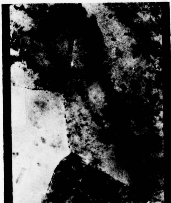
Figure 2. 7075 Al Alloy. Dark Band is Dislocation Debris. 30,000x
