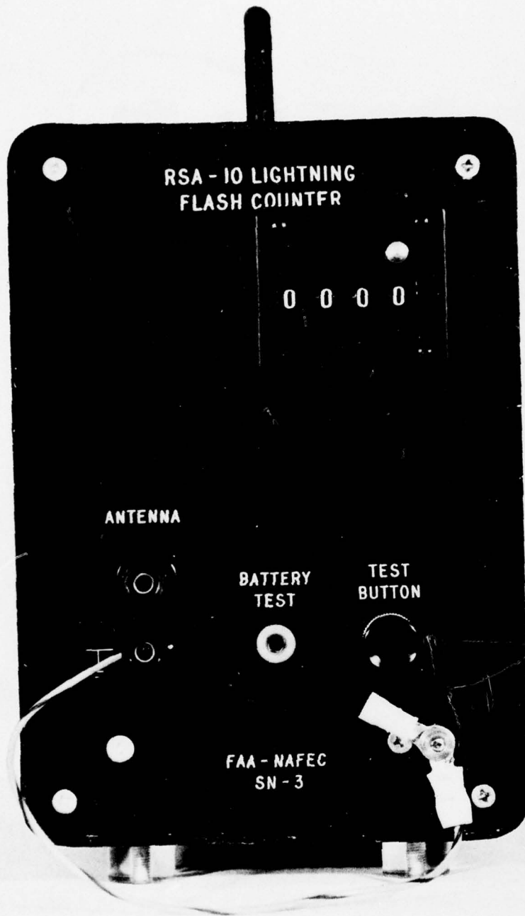
FIGURE 4. LIGHTNING-FLASH COUNTER SENSOR UNIT
