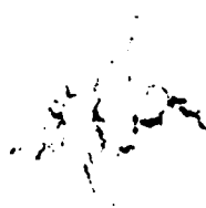
(b) SCRIPT-LIKE PATTERN OF PLANAR MICROFRACTURES
