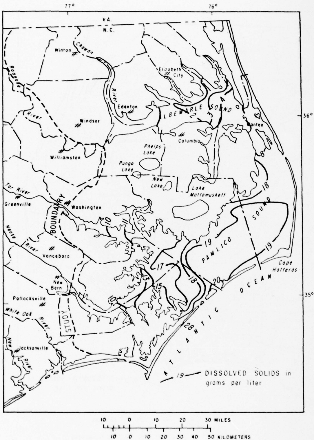
Figure 43.--Average dissolved solids in water in larger sounds of northeast North Carolina for the month of December. (Modified from Williams and others, 1967.)
