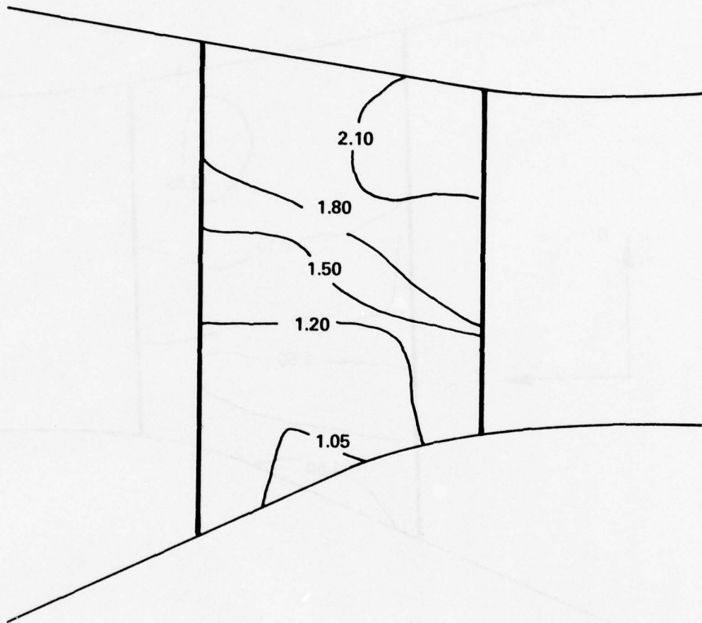
Figure 36. Suction Surface Ratio of Static Pressure to Inlet Total Pressure for ARL Rotor with Splitter, 100-Percent Design Speed
