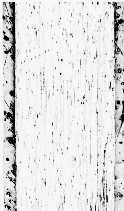
Figure 39: Steel Clad Laminate After Heat Aging (50X)
