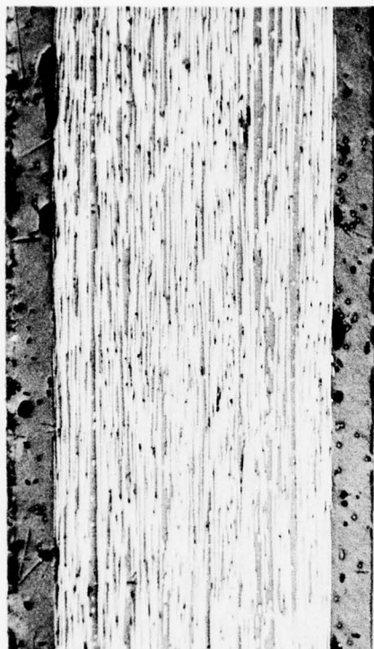
Figure 34: Aluminum Clad Laminate Before Thermal Shock (50X)
