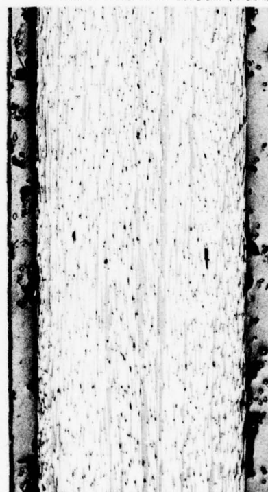
Figure 37: Aluminum Clad Laminate After Heat Aging (50X)
