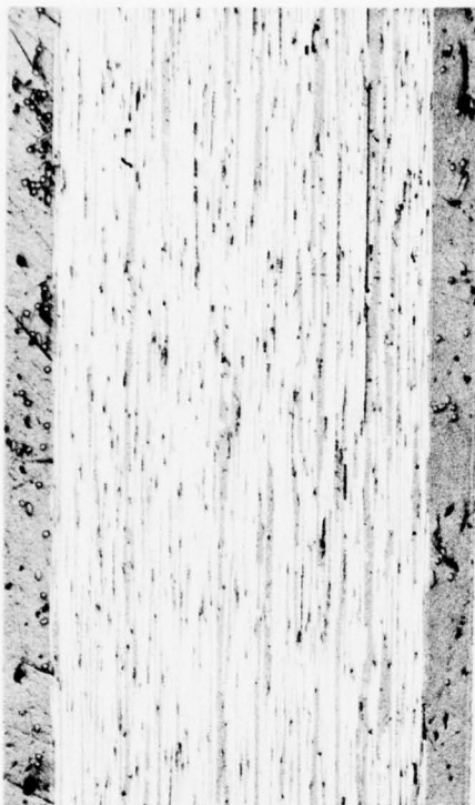
Figure 38: Steel Clad Laminate Before Heat Aging (50X)
