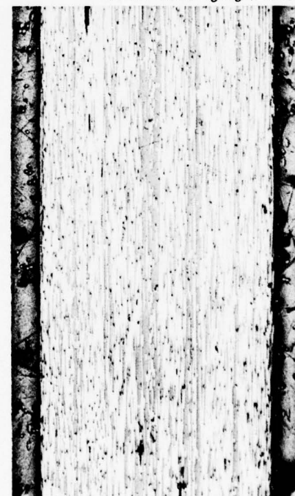
Figure 41: Steel Clad Laminate After Thermal Shock (50X)
