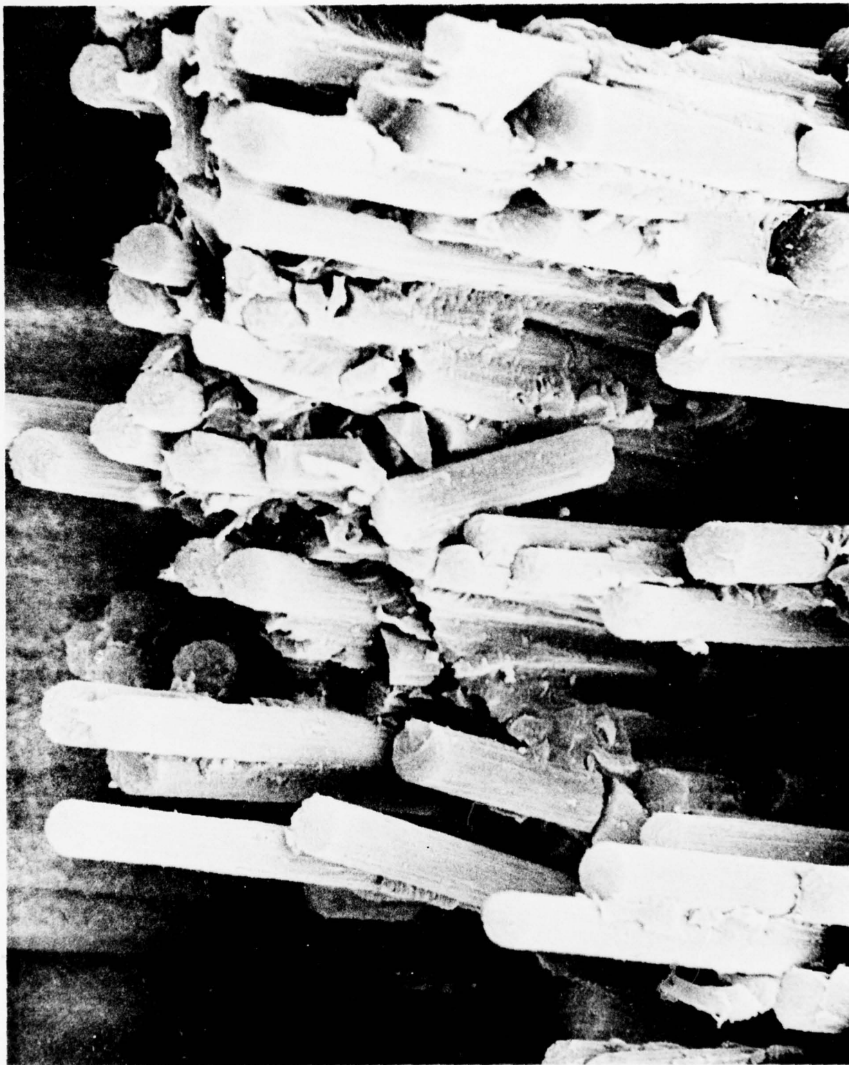
Figure 2: P-1700/A-S-Epoxy Unidirectional Graphite Composite (600X)
