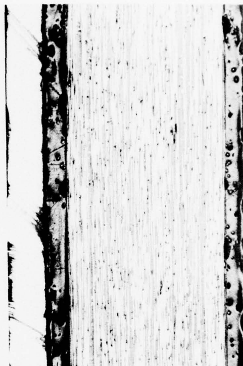
Figure 35: Aluminum Clad Laminate After Thermal Shock (50X)
