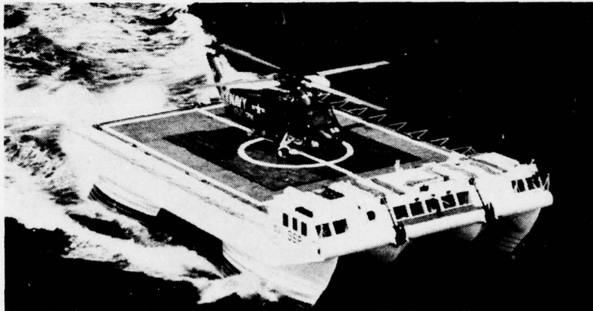
STABLE SEMISUBMERGED PLATFORM (SSP).
