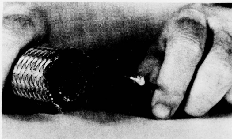
THE THIN, LIGHT FIBER OPTICS CABLE AT RIGHT REPLACES THE STANDARD CABLE AT LEFT.
