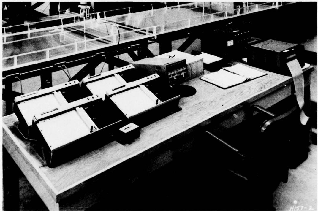
Figure 4. Instrumentation for measuring water surfaces and forces on moored tows
