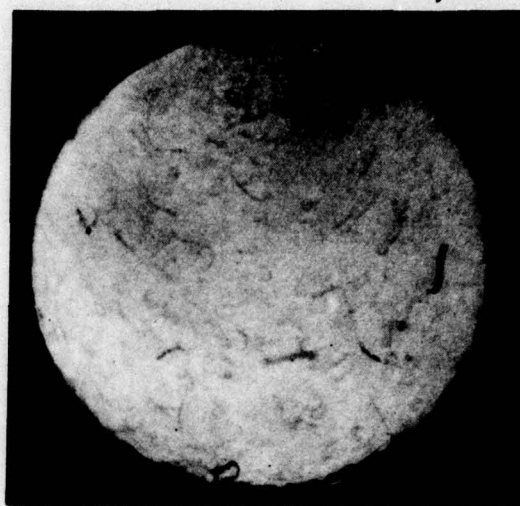
D. Large gate, medium speed, cold mould. Screw 52 r/min
