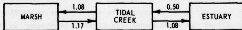
Figure 8. Tidal transport of nutrients between microcosm compartments. Units are in milligrams per day for nitrogen and phosphorus and grams per day for carbon
