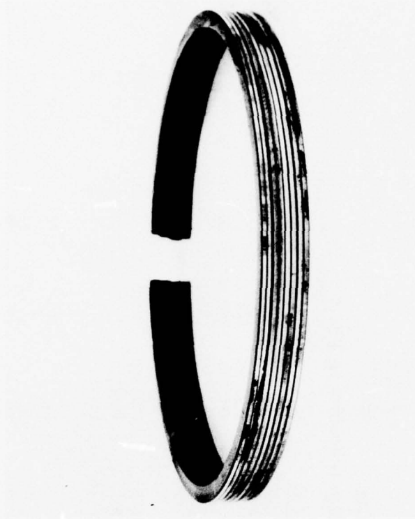
Unacceptable Test #4, High Sulfur Fuel
