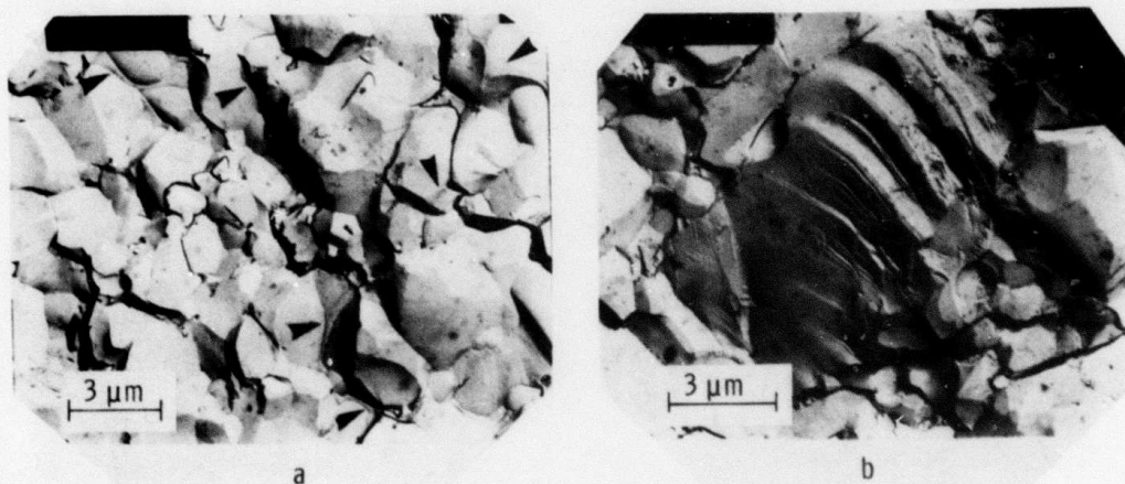
Figure 3-25. Replica Transmission Micrographs of 1115°F Fracture Surfaces - Norton Hot Pressed SiC (NC203)
