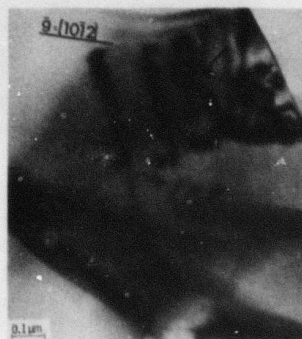
Figure 3-18. Dislocation Structure in HS130 Silicon Nitride a. 2 Grain \bar{g} = [0\bar{1}127] , [\bar{1}2\bar{1}1] ZA (100 kV) b. Near Dimples (arrow) in a \alpha Grain \bar{g} = [10\bar{1}2] , [\bar{1}3\bar{2}2] ZA (100 kV)
