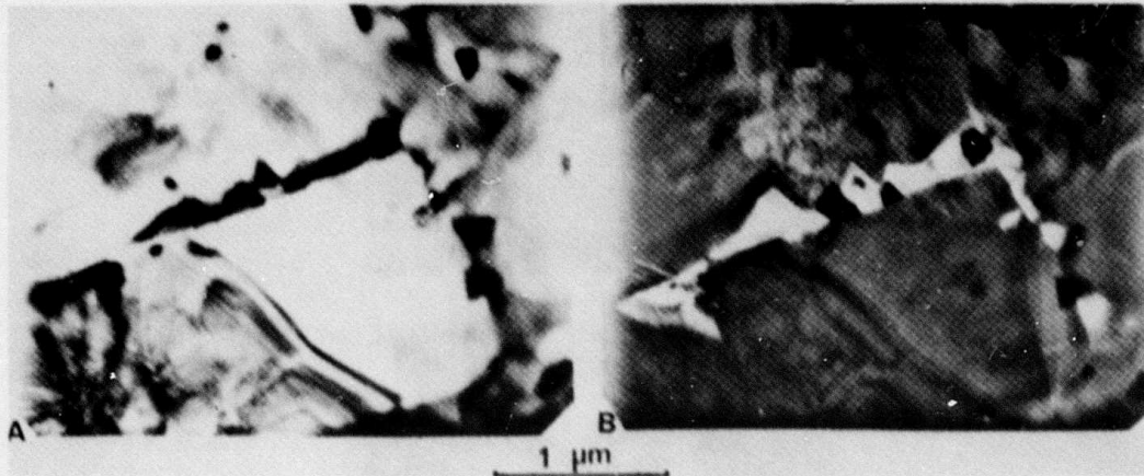
Figure 3-33. Transmission Electron Micrographs Showing Inclusions in Grain Boundaries of Hot Pressed SiC (NC203) A - Bright Field; B - Dark Field (1000 kV)
