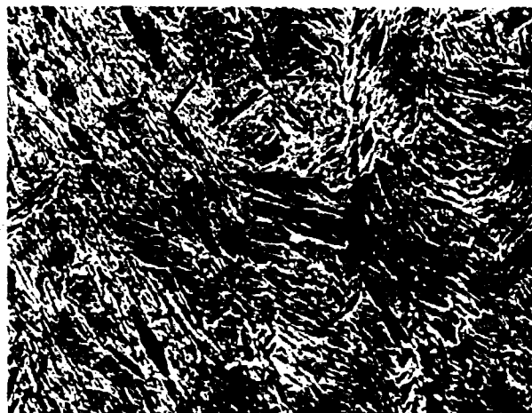
SECTIONED PERPENDICULAR TO RD 2 CROSS-ROLLED 60%
