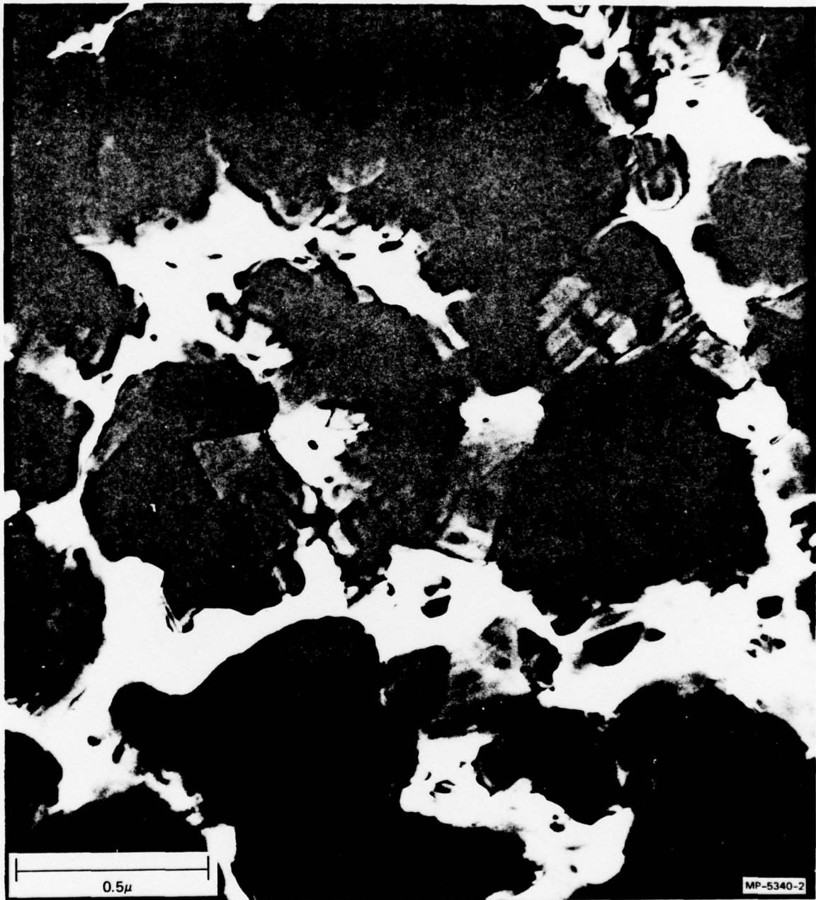
FIGURE 2. BRIGHT FIELD ELECTRON MICROGRAPH OF Au FILM EVAPORATED ON (100) SILICON AT SUBSTRATE DEPOSITION TEMPERATURE OF 150°C.
