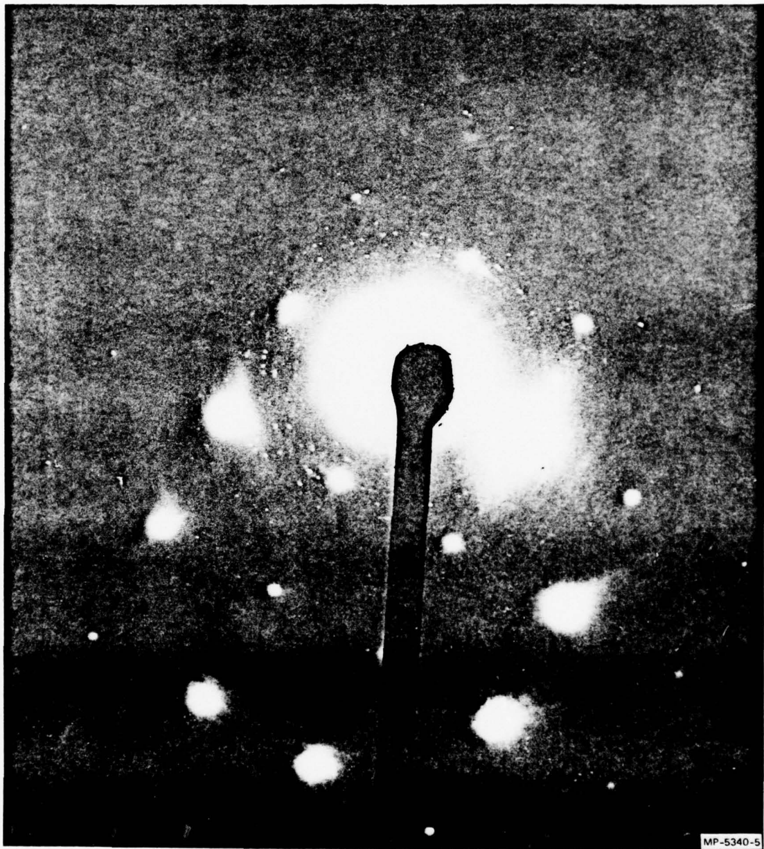
FIGURE 5. TRANSMISSION ELECTRON DIFFRACTION PATTERN OBTAINED FROM MIXING ZONE OF ANNEALED Au/Si STRUCTURE. SUBSTRATE DEPOSITION TEMPERATURE = 50^{\circ}\text{C} ; ANNEALED IN AIR FOR 12-HOURS AT 400^{\circ}\text{C} .
