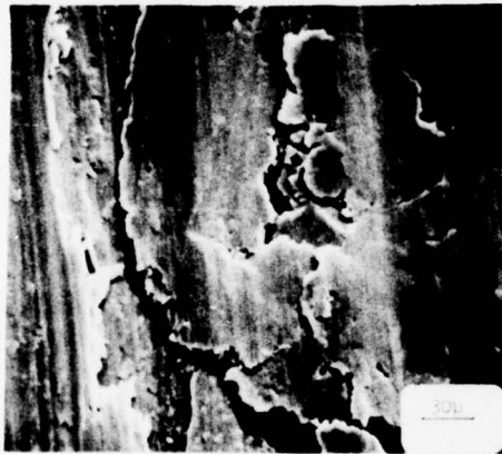
Figure 23: 2124; V = 17.5 fps; \sigma = 610 psi; N = 50,000
