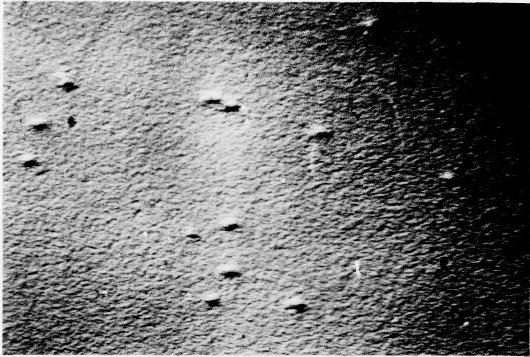
Fig. 22 — Gallium etched substrate surface oriented 3° off (100) → (110)
