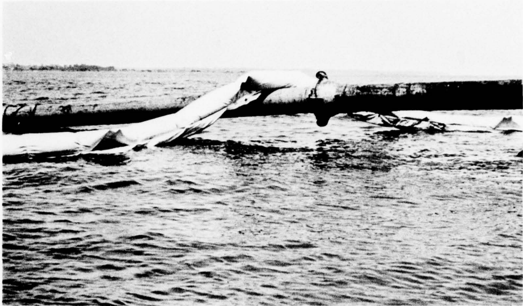
Figure 41. Curtain driven onto pipeline by storm at site 3
