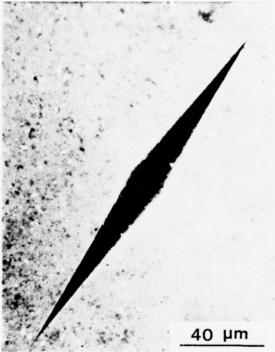
Figure 2. 2600-gm Knoop Indentation in HP Si 3 N 4 (a) Indentation on Polished Surface
