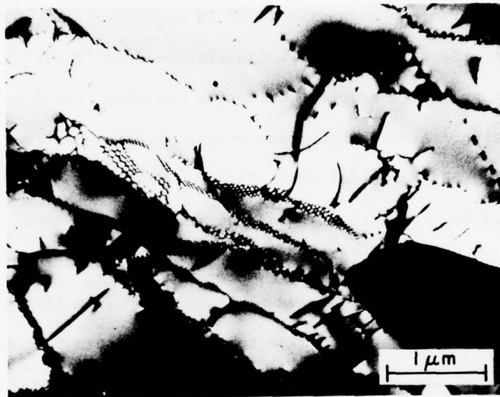
Figure 33. General Dislocation Substructure in Creep-Deformed Ti_3Al ( 800^{\circ}C , 20 ksi)
