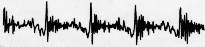
C) Residue inverse filtered signal from speech waveform.
