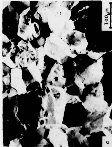
Fig. 10 - Micrographs of Alloy 718, Heat A, modified heat treatment; (a) optical micrograph of a polished and etched sample, (b) SEM micrograph of fracture surface after test at 427 deg C, (c) SEM micrograph of fracture surface after test at 539 deg C. Direction of crack growth was from left to right.
