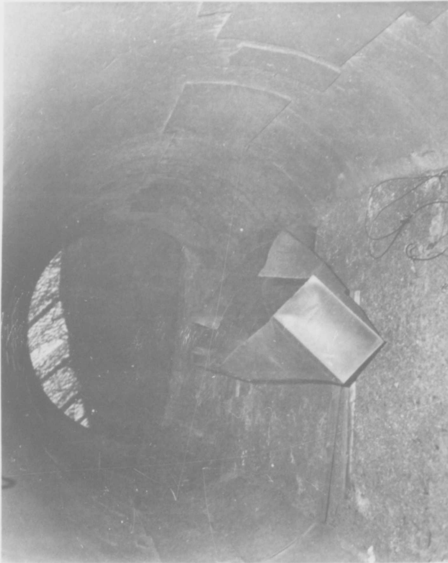
Figure 10. One-half scale test vessel at vent ratio of 1100, after test.
