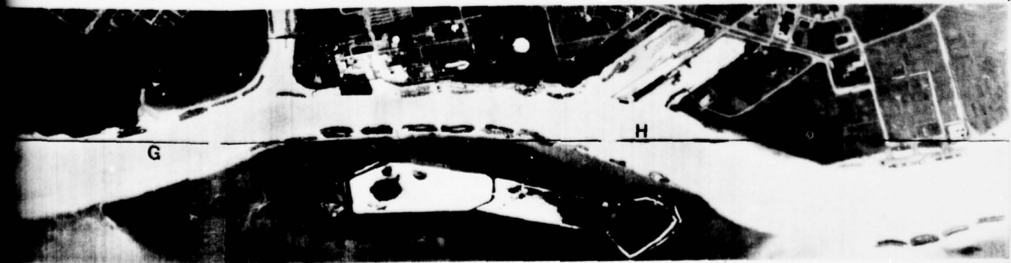
Figure 9 (cont'd). RS-14 thermal imagery with graph of PRT-5 radiation thermometer data. Warm features are lighter on the imagery. Note the occasional high temperature spike on the PRT-5 graph. This spike is probably caused by an electronic signal surge.
