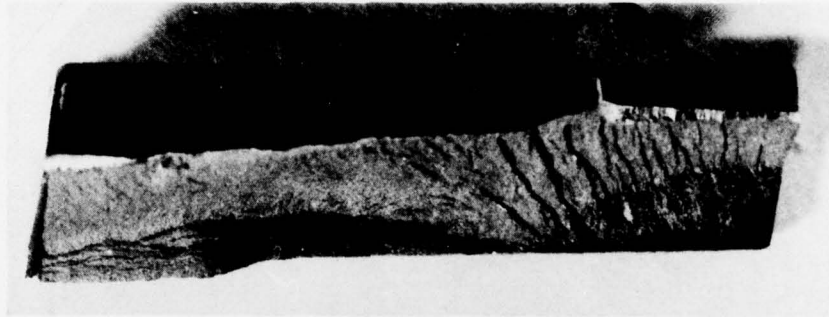
Fig. 10 — Typical fracture surface showing the three-dimensional characteristics of a fatigue crack
