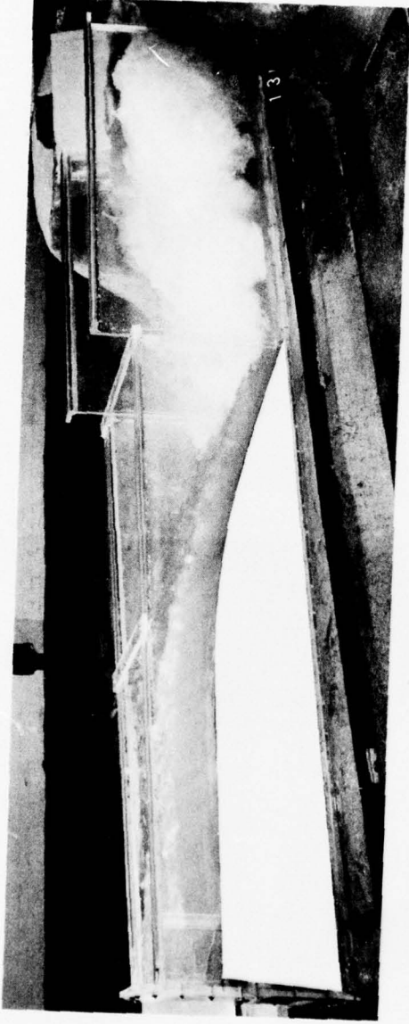
Photo 5. Flow conditions in stilling basin, recommended design; pool el 675, tailwater el 582.5, discharge 8,000 cfs
