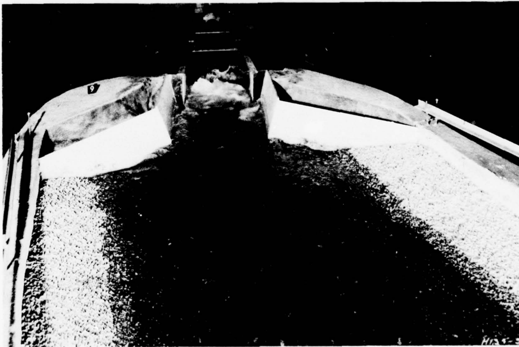
Photo 10. Flow conditions in exit channel, recommended design; pool el 675, tailwater el 580.5, discharge 5,000 cfs
