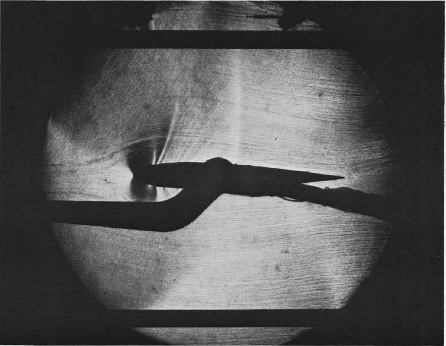
Figure 20 SCHLIEREN VIEW OF THE FLOW FIELD AT M_\infty = 0.80 , \alpha = 1^\circ , 6% BLOCKAGE. WALL CONTROL USED TO ESTABLISH THE LONGITUDINAL VELOCITY COMPONENTS
