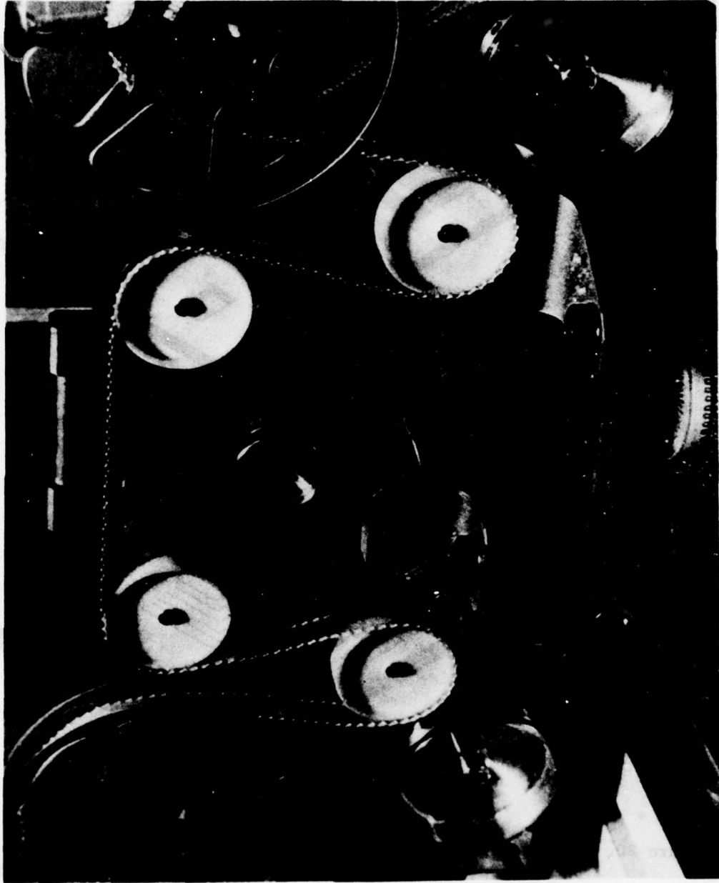
Figure 29. The TAB Tape Handler for the Automatic Electrical Testing of Tape-Mounted Integrated Circuits. (Courtesy of CII Honeywell Bull)
