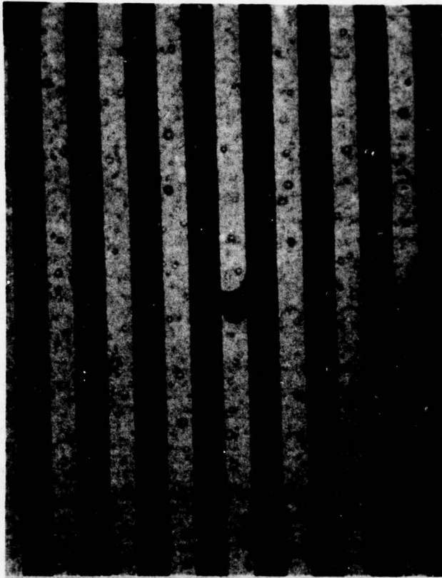
Figure 76. Aluminum Etch Defect in the Second MMI 5086 Chip Removed from S/N 2 Hybrid Assembly.
