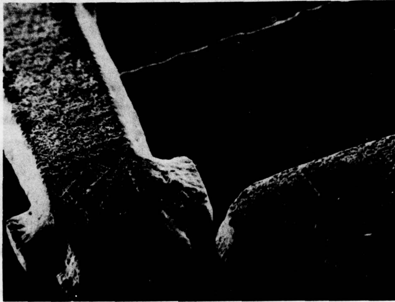
Figure 47. SEM View of Gold-Tin Fusion Inner Lead Bonds to Kovar TAB Leads Showing Good Fillet Formation. The Etch Factor of the Kovar is also Noticeable.
