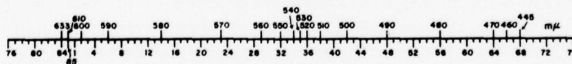
FIG. 9. Linear arrangement of Farnsworth selection of colors with appropriate spectrum wavelengths indicated.
