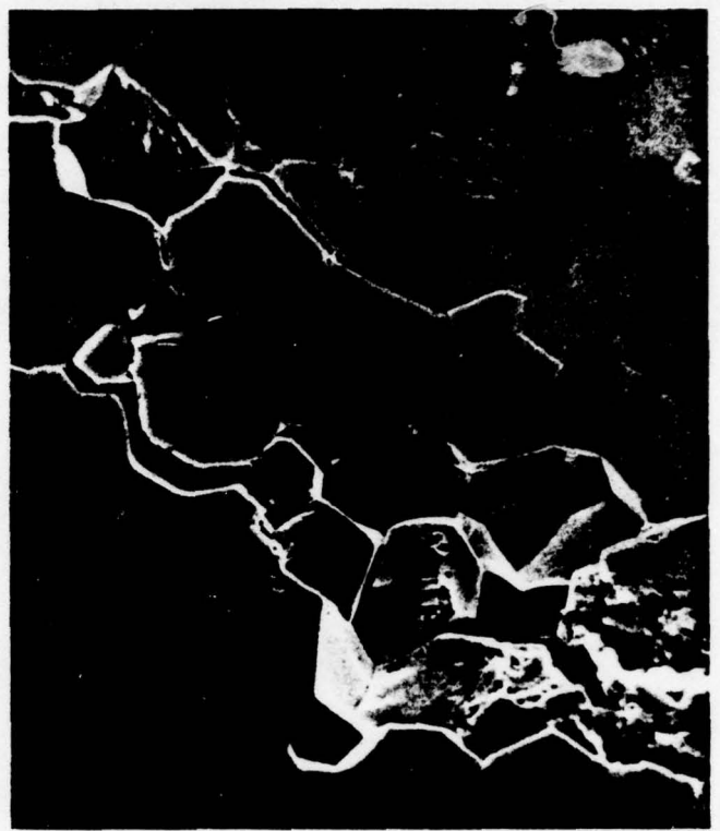
Figure 10. Intergranular cracking in Ti-5Al-5Sn-5Zr. 700X.
