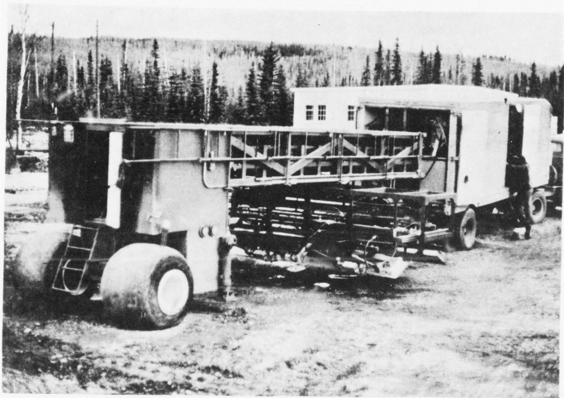
Figure 24 Prototype apparatus for applying polyurethane insulation to embankments.
