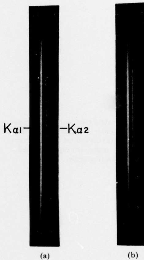
Fig. 4 — Resolution of K\alpha_1 K\alpha_2 doublet (Cu K\alpha , 3rd order) at crossover of curved ADP crystal. (a) Crystal set for maximum diffracted intensity, (b) crystal rocked through diffraction angle.
