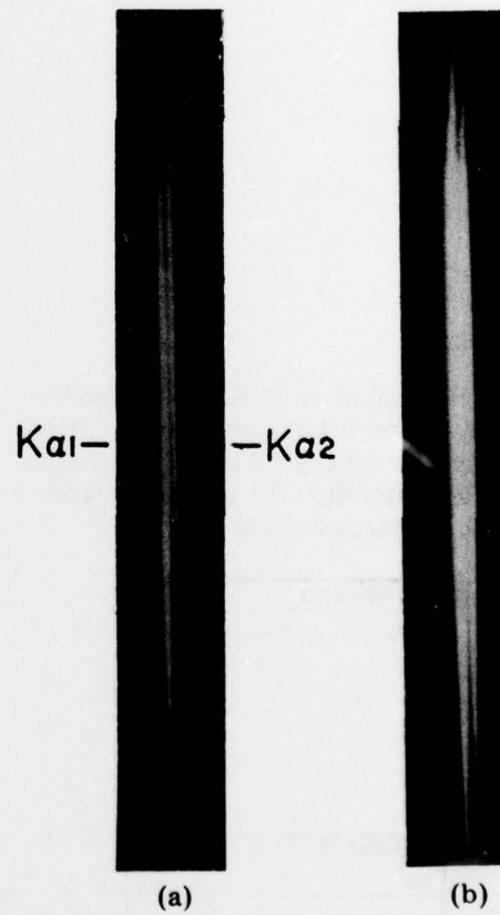
Fig. 2 — Resolution of K\alpha_1 K\alpha_2 doublet (Cu K\alpha , 1st order) at crossover of curved LiF crystal. (a) Crystal set for maximum diffracted intensity, (b) crystal rocked through diffraction angle.
