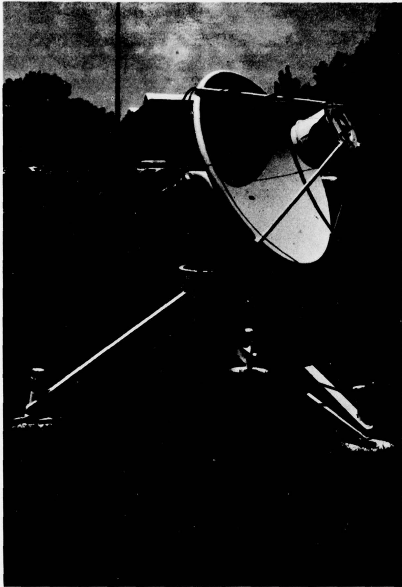
Figure 11. Minitracker Antenna and Pedestal
