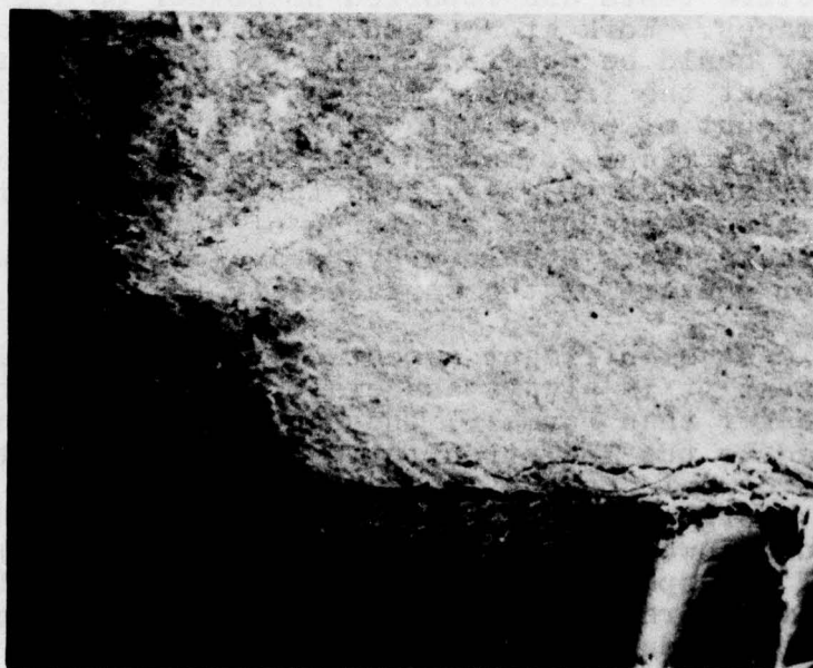
Fig. 1b — Failure from surface flaw x 50
