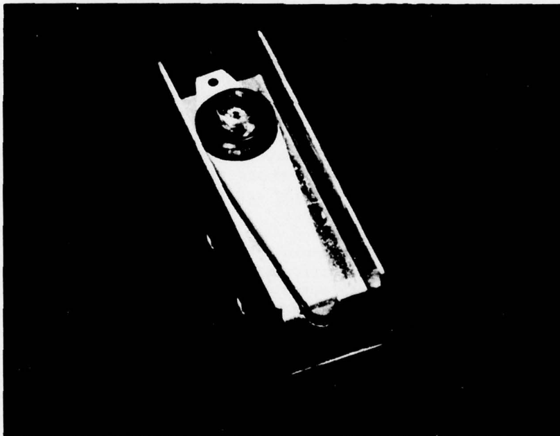
Fig. 1. Tunable semiconductor diode laser in standard package. Overall dimensions are 19.1 mm long, 6.4 mm wide, and 7.9 mm high. Typical laser length is 0.5 mm.
