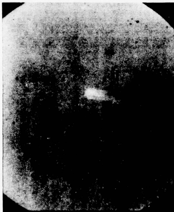
FIG. 3. Back-lighted micrograph of a 50- \mu m carbon particle taken 6 \mu sec after being hit by a laser pulse incident from the left.
